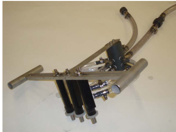
Filling handle with 3 nozzles for automotive batteries.
