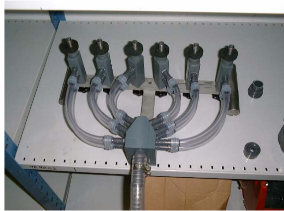
Filling handle with 6 nozzles for automotive batteries.
