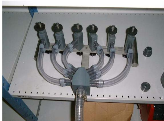
Filling handle with 6 nozzles for automotive batteries.
